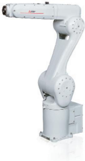
**Articulated** or jointed-arm industrial robots most commonly have six axes of movement. They are easier to align to multiple planes and can be redeployed with less difficulty. They can be used in a wide variety of applications including:
